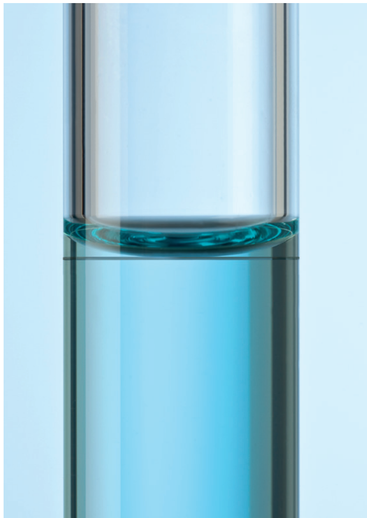
A typical surface curvature of the liquid level (meniscus)
