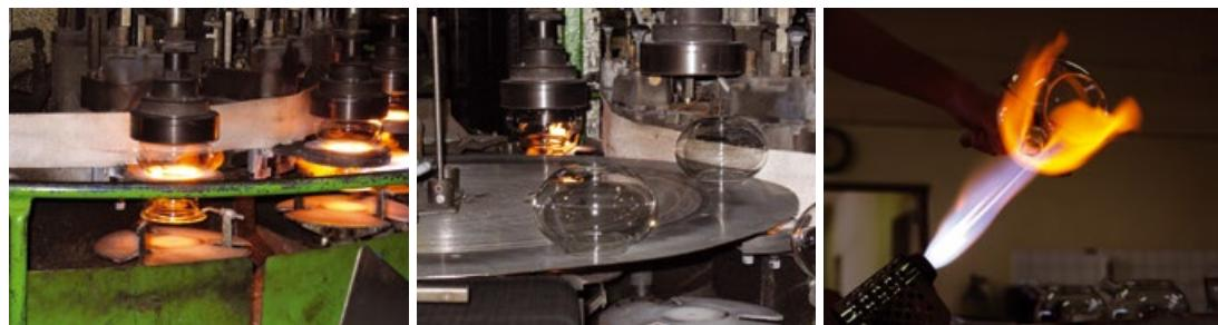
Heat-resistant glass for domestic use was produced in Jena for the first time in around 1920. By developing the borosilicate glass, Otto Schott created a universal material which, after laboratories and the industry, quickly conquered households as well.
